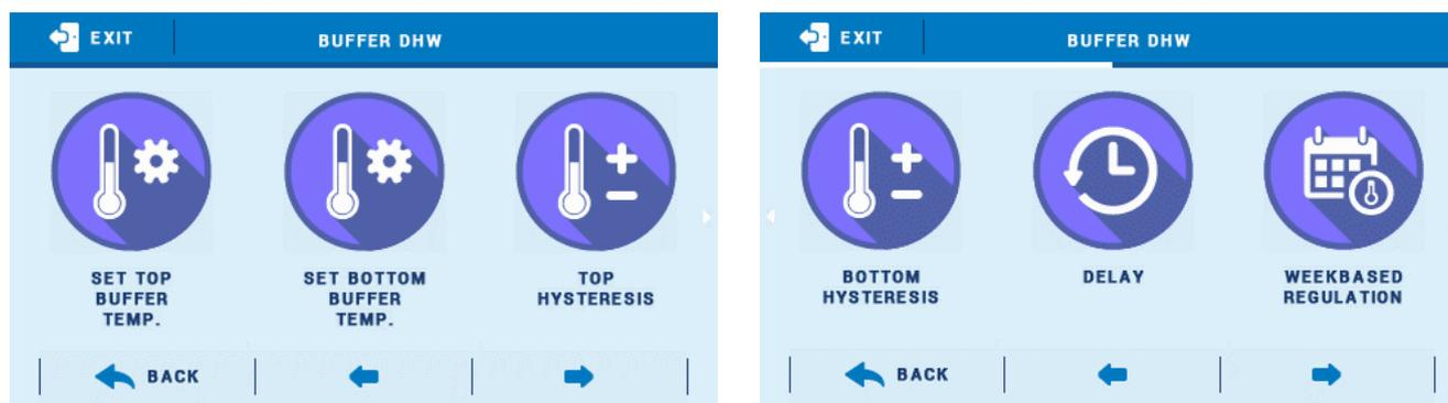
Moreover, the device may operate according to weekly program (described in detail in section 9), which controls the temperature of the upper sensor. The user may choose which sensors will serve as top and bottom sensors.
