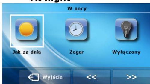
By selecting *At night* option the user enters the panel enabling him/her to adjust the screen view at night: *As at daytime*, *Clock* or *Switched off*. The selected screen view is activated during nighttime, after the screen has not been touched for 20 seconds. In order to return to the main menu, touch the screen.
