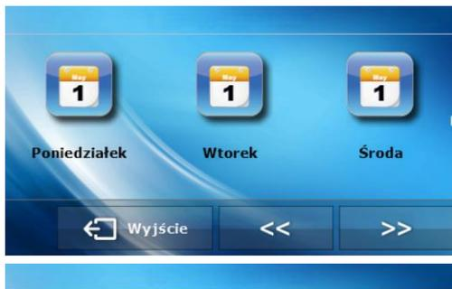
After selecting day of the week, the user sets the time when the device will operate. Using arrows the user selects the exact time of device activation and then chooses ON or OFF status. **Copy** button is used to copy a given status for subsequent hours.
