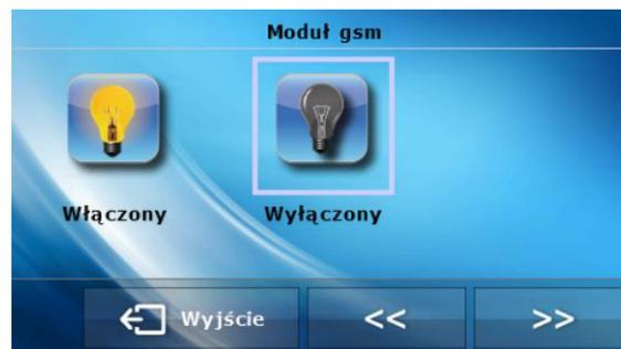
GSM Module is an optional device which, cooperating with the controller, enables the user remote control of the CH boiler operation via mobile phone. The user is sent an SMS each time an alarm occurs. Moreover, after sending a certain text message, the user receives feedback on the current temperature of all the sensors. Remote change of the set temperatures is also possible after the authorisation code is entered.
