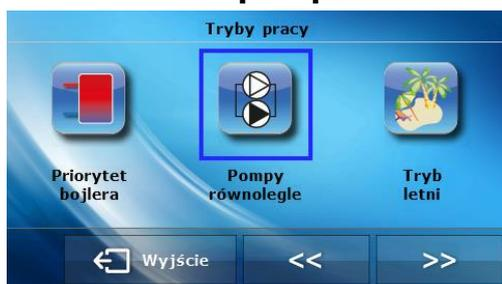
In this mode, all active pumps and valves operate simultaneously. The valves maintain the pre-set temperature and the water tank is heated to the pre-set temperature.
