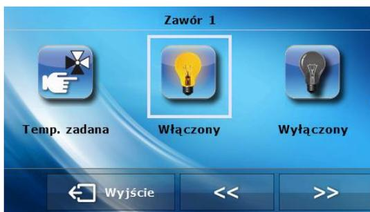
This option is used to activate valve 1. When the valve is turned off, the pump is also inactive. After connecting the controller to the power source, the valve is always calibrated, even if it is deactivated. It prevents the valve from remaining in dangerous position.
