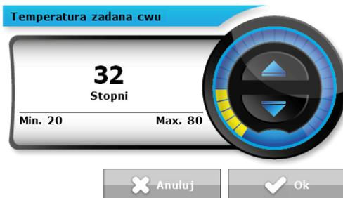
This function is used to adjust the pre-set temperature of domestic water. It may be done from the main screen view when *DHW* view is active. After the water in the water tank reaches this temperature value, the controller switches off the DHW pump. The pump is enabled again when the temperature drops below the set value minus *DHW hysteresis*.
