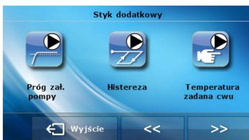
➤ **Activation threshold** – this option is used to set the temperature of device activation. When the temperature is below the set value, the device is inactive whereas when the temperature exceeds this value, the device is enabled and operates until the set temperature is reached.
