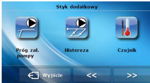
➤ **Activation threshold** – this option is used to set the temperature of device activation. When the temperature is below the set value, the device is inactive whereas when the temperature exceeds this value, the device is enabled.
