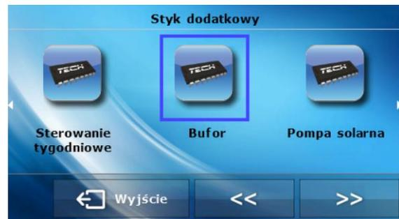
**Example:** The controller is used in CH boiler system with 3 valves. The system includes a heater connected to additional contact (*Heating need* function). Pre-set temperature of the valves is 50 °C. *Heating need* function operates using information provided by CH sensor. When the CH boiler temperature drops below 50 °C (CH boiler is not able to increase the temperature to the pre-set value), the controller activates the heater.
