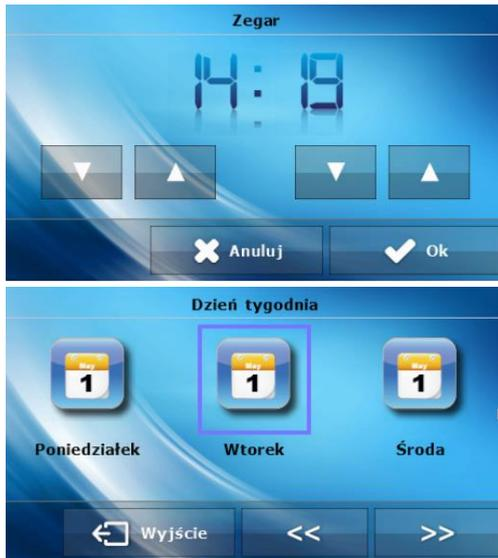
Using *up* and *down* buttons the user may set hour and minute.
