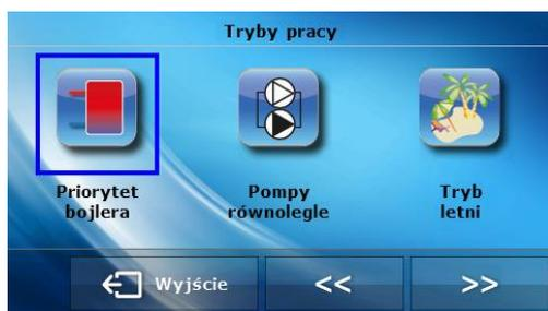
In this mode, the DHW pump is activated first and it operates until the pre-set DHW temperature is reached (the valves close completely and the valve pumps are switched off). After the set temperature has been reached, the pump is switched off and the mixing valves are activated (along with the pumps – according to their settings).
