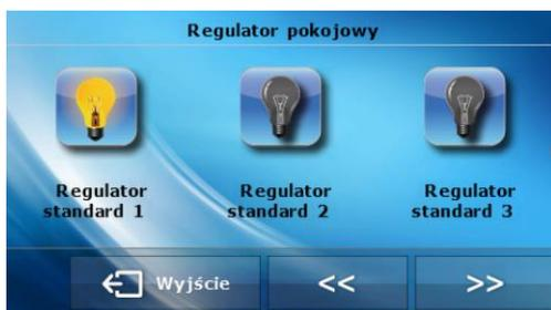
It is possible for the additional device to work according to the signal from the maximum of 4 room regulators. Then, the device will switch off only when each of the regulators signals that its pre-set temperature has been reached.
