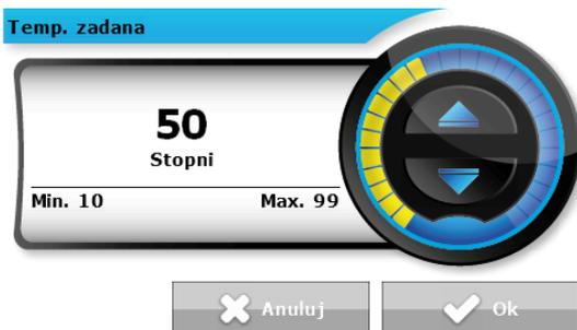
This option is used to set the desired temperature which will be maintained by valve 1. The temperature may also be adjusted directly from the main screen, when *Temp 1* is active. During proper operation, the temperature of water behind the valve approaches the pre-set temperature of the valve.
