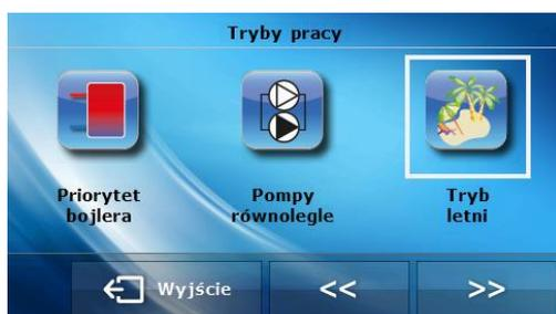
In this mode, the **CH valves** are closed to prevent unnecessary house heating. In case the CH boiler temperature is too high, the valve is be opened as an emergency procedure ( it requires activation of return protection!)
