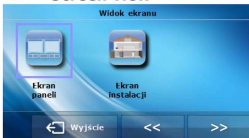
With this function the user can change the screen view switching between *panel screen* and *installation screen 1* or *2*. All screen views are described in part V.b. The setting applies during daytime.
