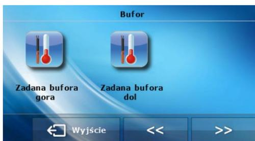
**Pre-set buffer temp. top** – this function enables the user to define the pre-set temperature for the upper part of the buffer (sensor should be placed in the upper part of the tank). After this value is reached and the delay time elapses, the pump is disabled
