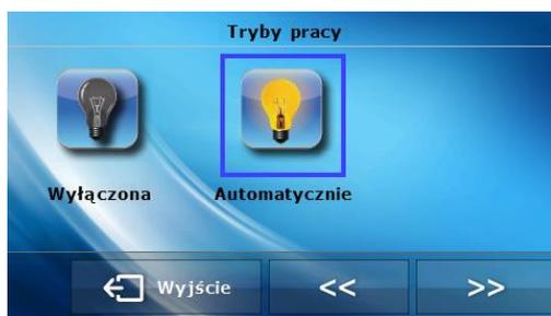
This function enables the user to switch off the DHW pump if it is not used, or to activate automatic operation mode (the pump operates according to parameters described in the following section) or heating mode (the pump operates when the sensor temperature is lower than the pre-set value, regardless of DHW pump activation threshold).
