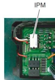
Spread the heat dissipation compound on the other side of IPM when you exchange Main PCB by the repair.
