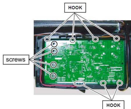
Remove the 4 mounting screw and hook.
