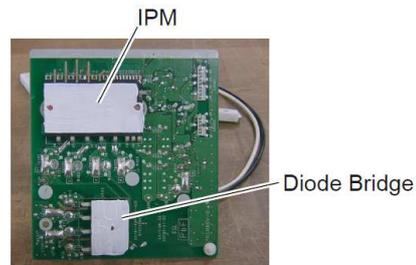
Spread SILICONE GREASE G746 evenly on the other side of the Diode Bridge and IPM when you exchange the Transistor PCB assy.
