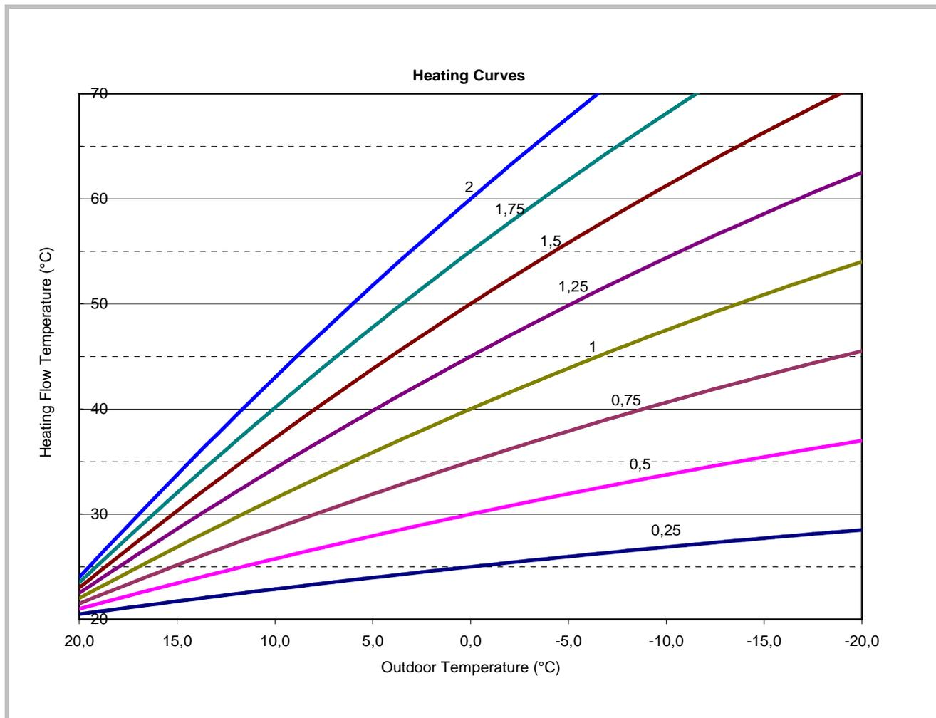
**Heating curve displacement**
