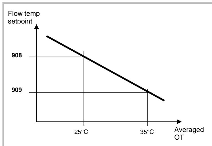
The cooling characteristic is adjusted for a 25°C room temperature setpoint. If the room temperature
