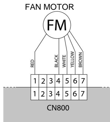
If the voltage is incorrect, replace Main PCB.
