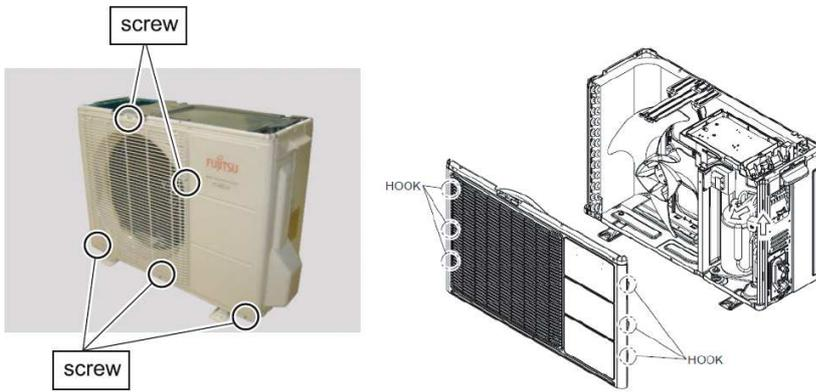
Remove the mounting screws.
