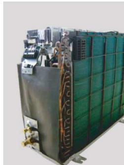
Remove the CABINET RIGHT ASSY by sliding upward.
