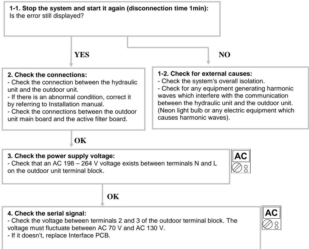
**Clear 4: Heat pump capacity signal error**
