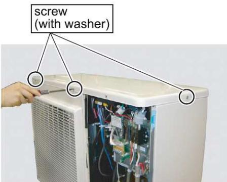
Remove the mounting screws.
