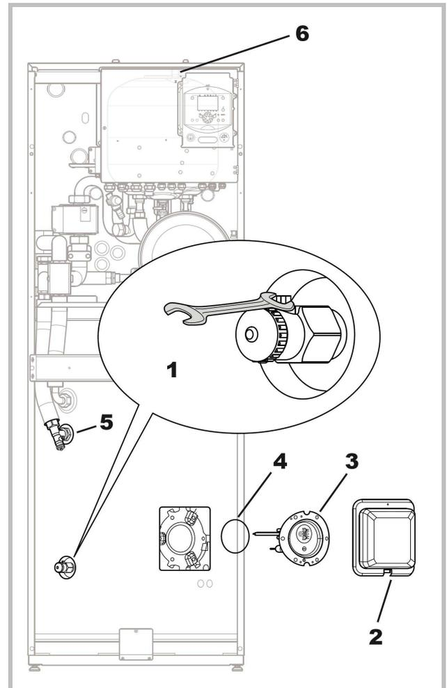
Figure 3 - Emptying the hydraulic unit and/or DHW tank
