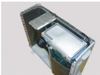
Remove the INVERTER BOX COVER by sliding upward.
