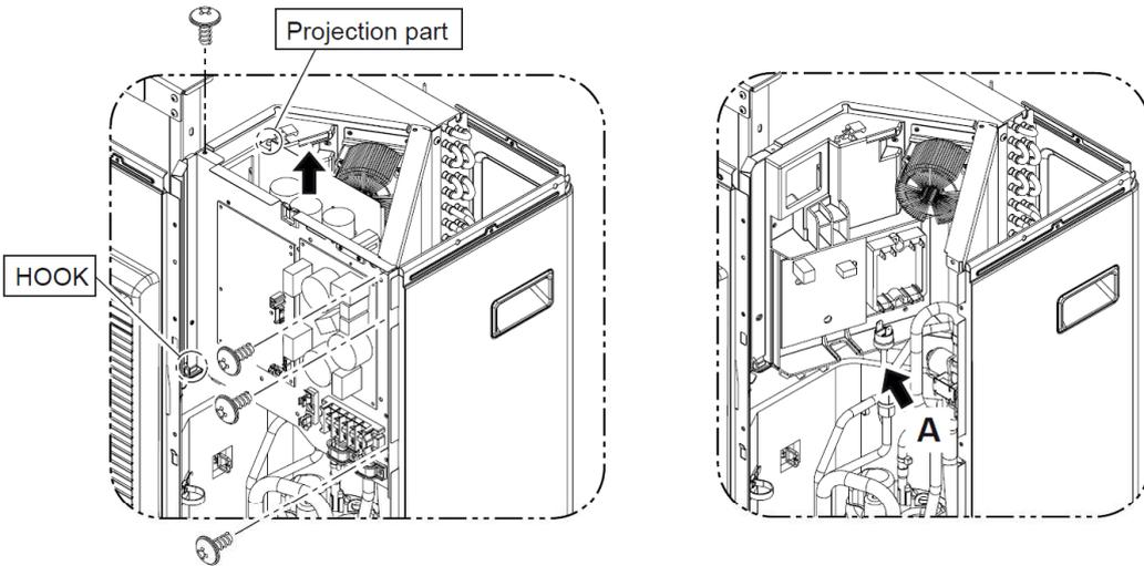
Remove the 4 mounting screws.
