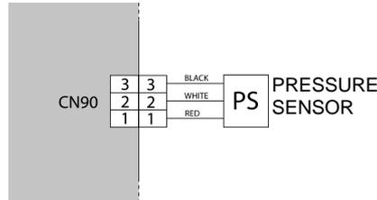
If the voltage is not correct, replace Main PCB.
