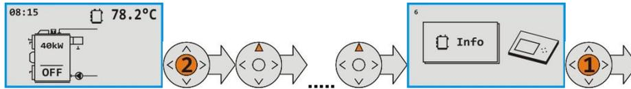
By means of the **ENTER** button we can display the current software version of the AK6000D module:
