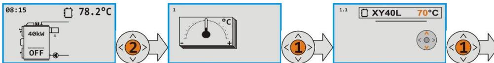
Basic view goes to the frame 1 where we use short click on the **ENTER** and we are in the frame 1.1. Short click of the **ENTER** and we can set required temperature by buttons ▲ or ▼ in **70 – 85 °C** range. Short click of the **ENTER** confirms choosed value and frame 1.1 we leave by double click of the ► (ESC).
