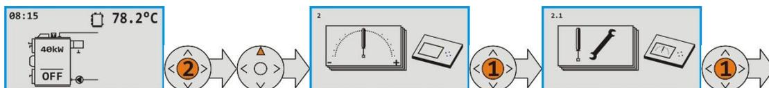
Basic view goes to the frame 1 where we use button **▲** till we get to the frame 2. Short click on the **ENTER** and we are in the frame 2.1. One more time click on the **ENTER** and we get to the frame 2.1.1. Using buttons **▲** or **▼** we can choose required parameter:
