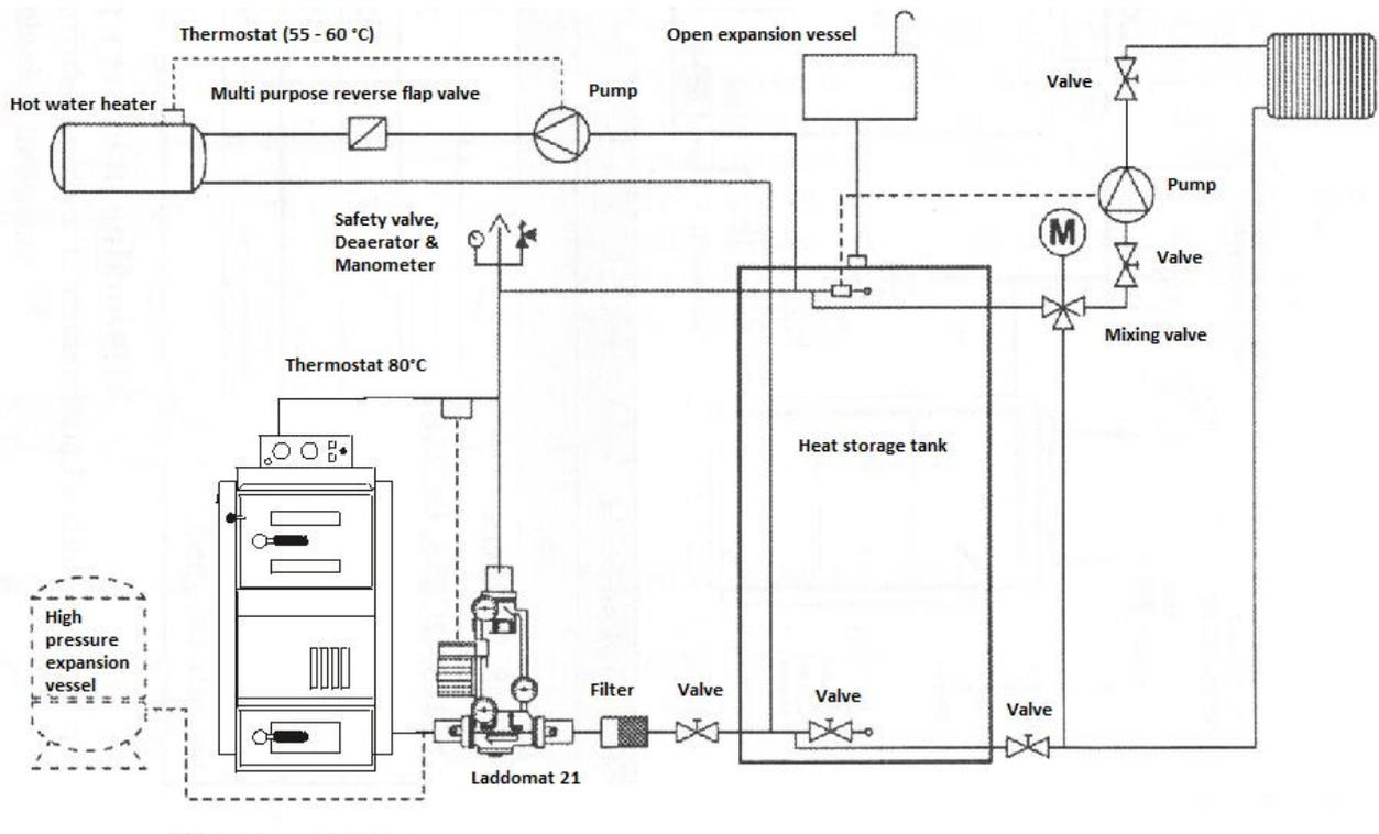
**Boiler Installation/Connection with a Heat Storage Tank**
