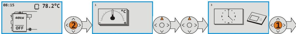
Basic view goes to the frame 1 where we double use button **▲** till we get to the frame 3. Short click on the **ENTER** and we are in the frame 3.1. Using buttons **▲** or **▼** or **ENTER** we can make required parameter to flash. Using buttons **▲** or **▼** we set flashed value to required time or date. Choice is stored by the **ENTER** and so we move to next position we want to change. Frame 3.1 we can leave by double click of the **▶** (ESC).
