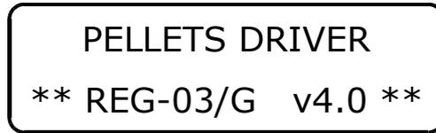
While activating, the burner carries out a test of the connected sensors. In case of one lacking, on the screen appears an appropriate message (---). The work of the burner without a heating water temperature sensor (CH) is blocked and an emergency mode is activated (CH pump is still on).
