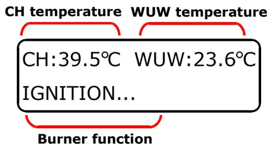
The burner may work in three working modes ("STOP", "IGNITION", "AUTOMATIC WORK"). The mode changes when the "MODE/↻" button is pressed. Activating the "STOP" mode is possible in all modes after pressing the "MODE/↻" button for 3 seconds. When Stop is activated, the burner goes at "Burning off" process (if there is fire) and the at "Cleaning" process.
