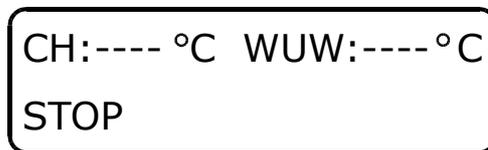
Correct connection of sensors causes displaying of actual CH furnace's temperature and the temperature of useful warm water of the WUW buffer (if the function is active). On the screen appears which function is currently used by the driver.
