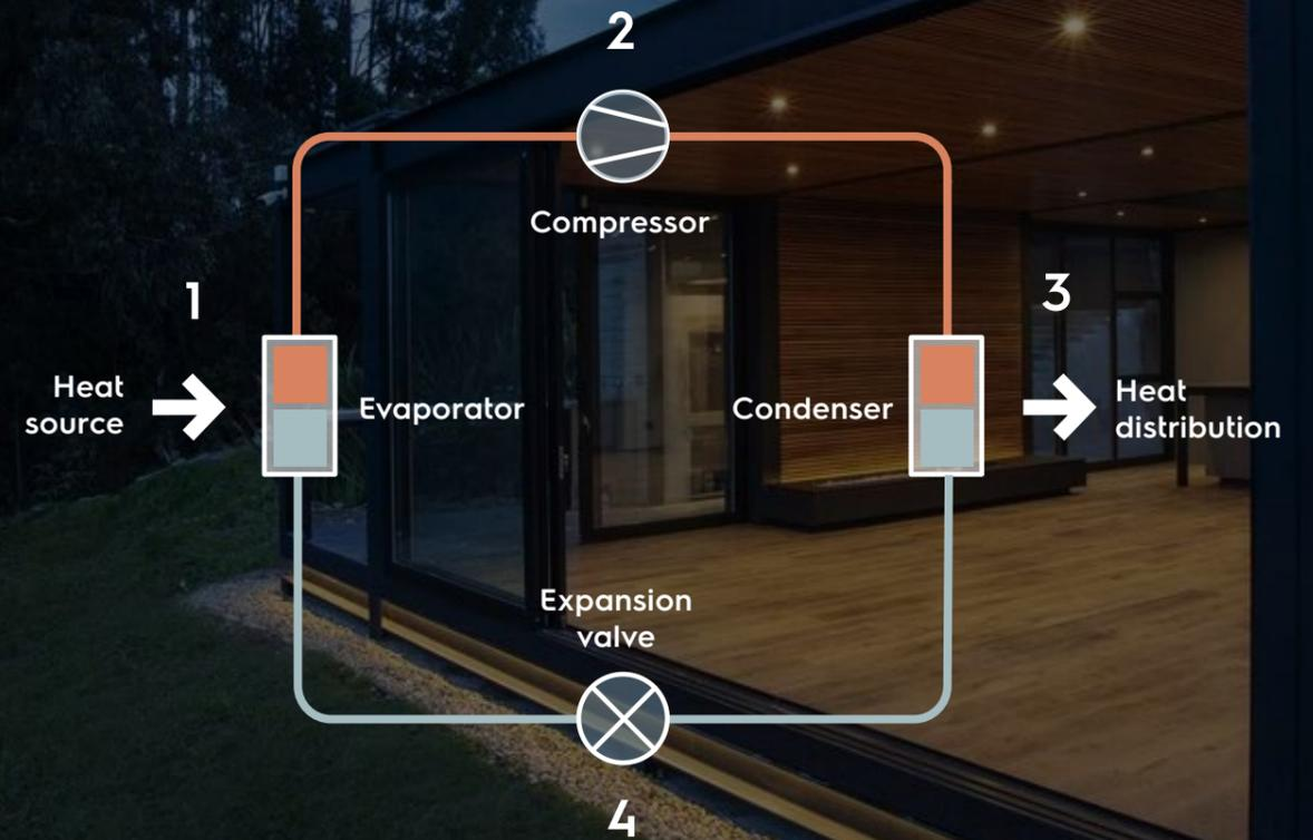
**1** The liquid refrigerant passes through the heat exchanger-evaporator, in which, due to the heat supplied to it from the outside air, its phase transformation into superheated vapor occurs. In other words, it evaporates like water in a boiling kettle.
