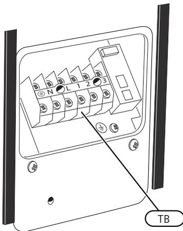
Communication is connected on terminal block TB. See also electrical wiring diagram on page 56.
