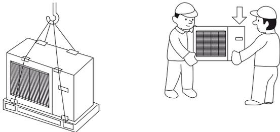
If AMS 10 needs to be transported across soft ground, such as a lawn, we recommend that a crane truck is used that can lift the unit to the installation location. When AMS 10 is lifted with a crane, the packaging must be undamaged and the load distributed with a boom, see the illustration above.
