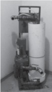
Flushing unit (or purging cart)
