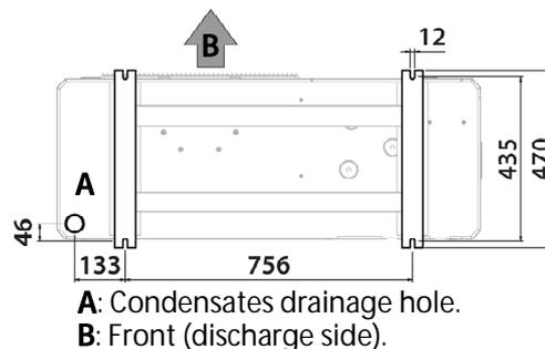
Preferably install the device in a well-drained place. To do this, it is advisable to provide a bed of gravel, sand or similar materials below said hole. If the drain hole of the heat pump is covered by a mounting base or by the floor, lift the unit to leave a free space of at least 100 mm below it.
