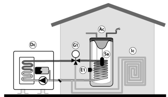
In addition, optionally, a backup heater (**E1**) can be installed, by means of what DHW temperatures higher than 50 °C can be obtained.
