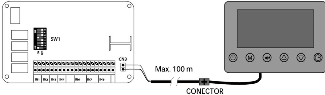
The cable supplied with the heat pump is 5 meters long. If necessary, it can be extended to a maximum distance of 100 meters (section between 0.5 ÷ 1.25 mm<sup>2</sup>).
