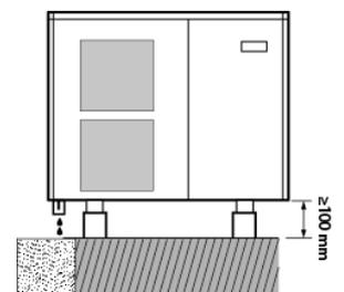
If it is installed on a terrace or façade, the condensate outlet must be led to a drain to avoid inconvenience and/or damage caused by the dripping of condensate water. If the installation is carried out in a region where the temperature can be below 0 °C for a long period of time, check that the presence of frost does not represent any danger.
