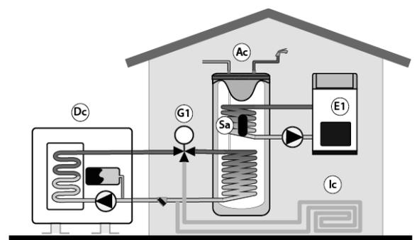
To perform the electrical installation of the DHW tank sensor, the 3-way valve (**G1**), and the backup heater or boiler (**E1**), read the "*Electrical Connections*" section of this manual carefully.
