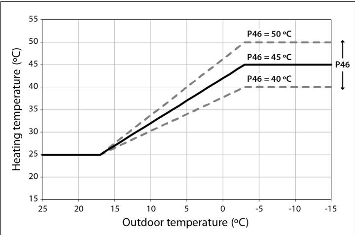
**NOTE: An incorrect adjustment of these operating curves may cause the heating installation not to generate the desired comfort in the home, failing to provide heating in extreme weather conditions of cold and/or causing overheating in hot weather conditions.**
