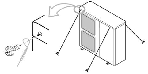
The device must be sufficiently accessible for subsequent installation and maintenance work. Make sure that the passage of the hydraulic and electrical connections to the interior of the house is possible and comfortable. The spacing measures indicated in the figure above are those strictly necessary to ensure correct operation of the device; however, sometimes, it will be essential to provide more space for maintenance work.
