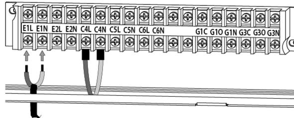
The relay that activates the heater has a maximum capacity of 20 A of consumption. Therefore, to connect resistors exceeding 4,500 W, a contactor must be interposed between the terminals of the power terminal and the heater.
