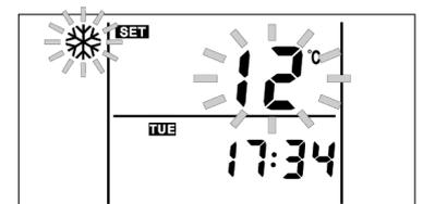
For the correct adjustment of the appropriate value of this operating mode, the recommendations of the installer or official Technical Service of **DOMUSA TEKNIK** should be followed. Depending on the type of installation, the location (climatic zone) and the relative humidity of the home,
