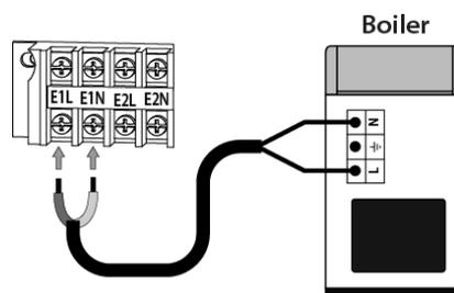
**NOTE:** When the backup source of energy is connected, it has to be taken in account that the maximum capacity of E1 relay is 20 A.
