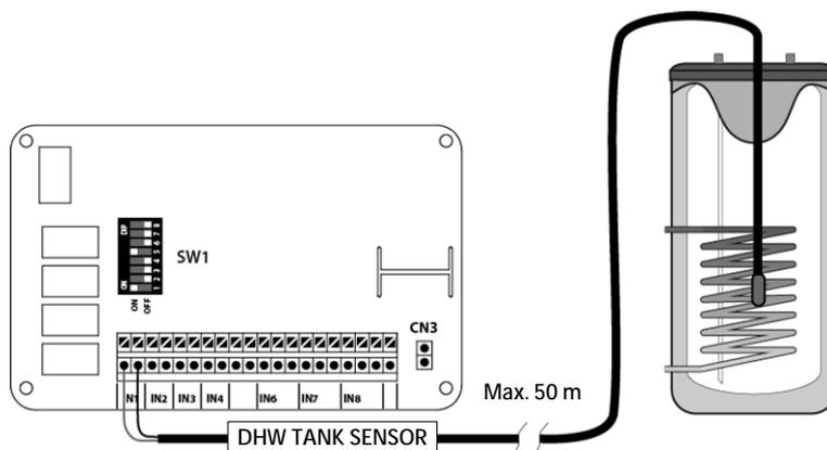
The sensor supplied with the heat pump is 5 meters long. If necessary, it can be extended to a maximum distance of 50 meters (section between 0.5 ÷ 1.25 mm<sup>2</sup>).
