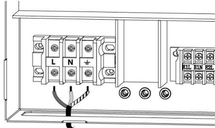
The dimensioning and type of the main supply cables must at all times comply with the rules and regulations in force. Nevertheless, the following table details some recommended features and dimensions, as a guide:
