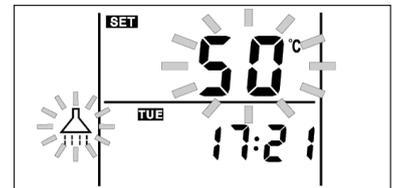
If the desired temperature in the tank is higher than 50 °C, it is essential to install an auxiliary heat source in the tank (electric heating resistor, auxiliary boiler, etc.). The **DUAL CLIMA** heat pump will heat the water in the tank to 50 °C and, from this temperature, activate the auxiliary source to reach the desired upper temperature.
