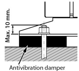
The receiving surface of the device must:
