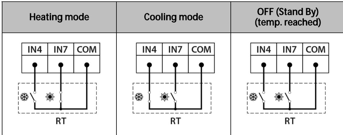
The **IN4** and **IN7** terminals are supplied from the factory with a jumper between each of them, so it will be necessary to remove **both jumpers** before connecting this type of room thermostat, as it is described in the following diagram. To disconnect the jumpers and connect the thermostat, **press** the upper screws with a thin flat screwdriver to release the cables and stop pressing to reattach them.
