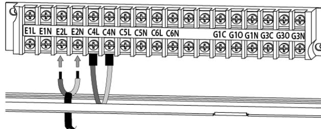
The relay that activates the electrical heater has a maximum capacity of 20 A of consumption. Therefore, to connect a heater exceeding 4,500 kW, a contactor must be interposed between the terminals of the power terminal and the heater.
