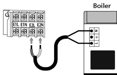
**NOTE:** When the backup source of energy is connected, it has to be taken in account that the maximum capacity of E2 relay is 20 A.
