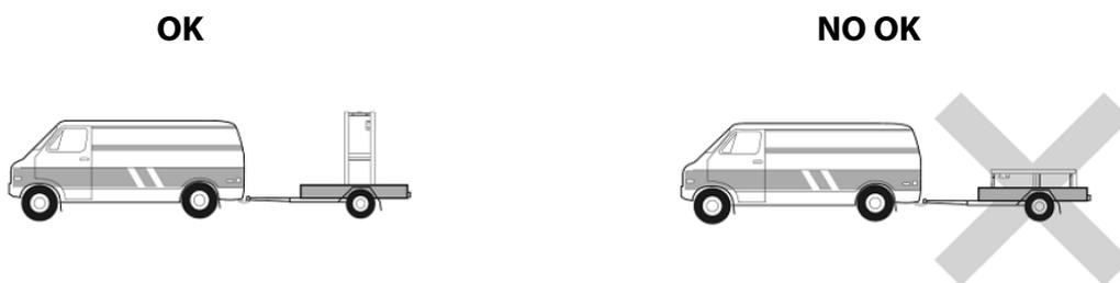
The heat pump packaging has a **"tilt indicator"** label to ensure that the machine has not been overturned during transport and storage. **Before receiving the machine from your supplier (distributor), check the status of this indicator and refuse the device without unpacking it if the warning switch of the label indicates that it has been overturned.**
