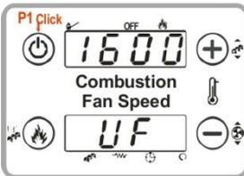
**UF**= Combustion Fan Speed [RPM/Volt]
