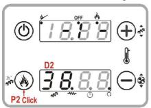
Click button **P2**: the display **D2** blinks. With other click of the button **P2** the power is changed according to the values.
