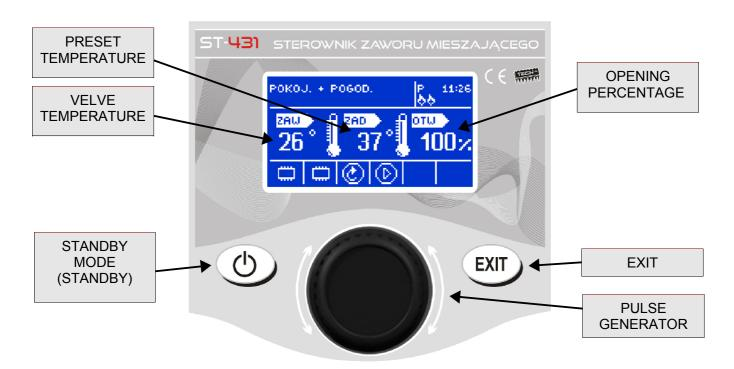
The principle of operation of the controller to valve servomotor is based on mixing feed circulating warm water with water returning from the heating circulation, in order to set the desired temperature and maintain it all the time at the same level.
